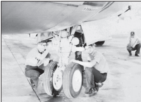
"Fig" and the crew inspecting after a hard landing — blown nose gear seal...
