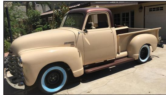
The original paint was stripped down to the base steel, primed and repainted with a classic look.
